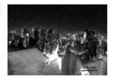
Available vacancies: Novel mesoporous titania thin films can be prepared with highly ordered vertical channels. Most of the pores are accessible from the film surface, and these channels can be filled with gold to produce gold nanowires.
